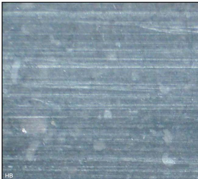
C120 = medium, visible grinding marks, pale colour, texture visible, grinding marks are visible in raking light.
