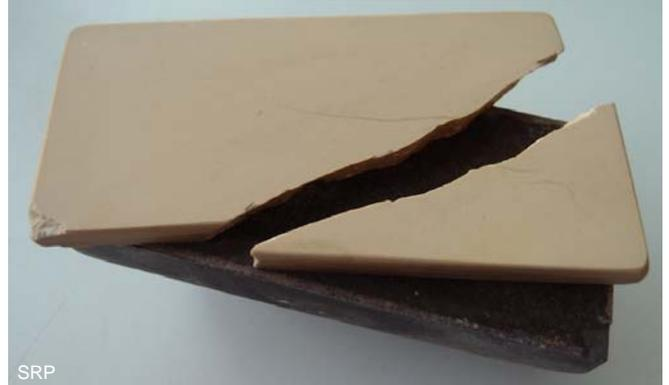
*These broken coticule can be repaired virtually invisible by gluing carefully.*
