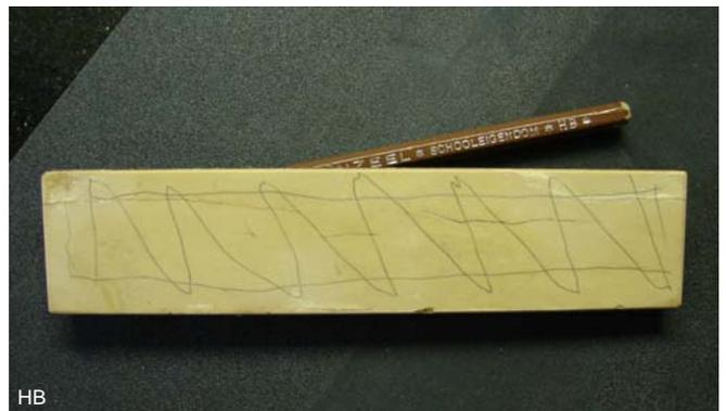
With pencil is a grid drawn on the stone. This allows us to verify the surface of the stone indeed has become flat.
