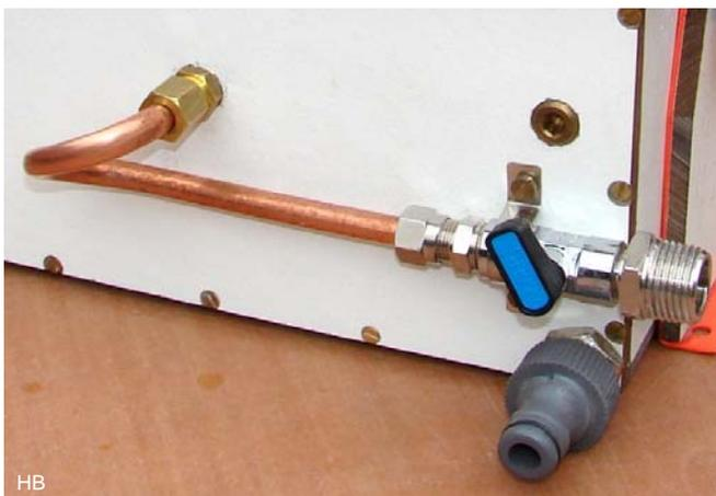
The water is provided by a 12 volt pump. The yield is too much and can be limited by the mini ball valve. The connections are 1/2 "gas thread so ordinary garden hose can be used which makes connecting and storing easy.
