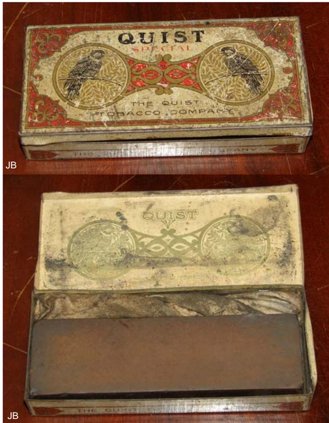
Usually artificial stone with an open character so the stone can absorb the oil.
