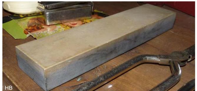
Rectangular stone usually in a box used to sharpen chisels on a workbench. The name is also used for other rectangular grinding- and whetstones.
