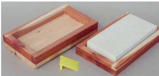
Simple construction of cedar. The stone is loose.
