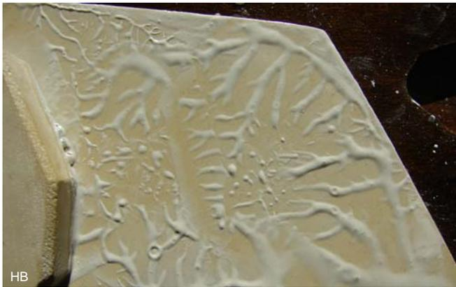
*Coticule slurry is milky white to light brown. The dark slurries grind faster.*
