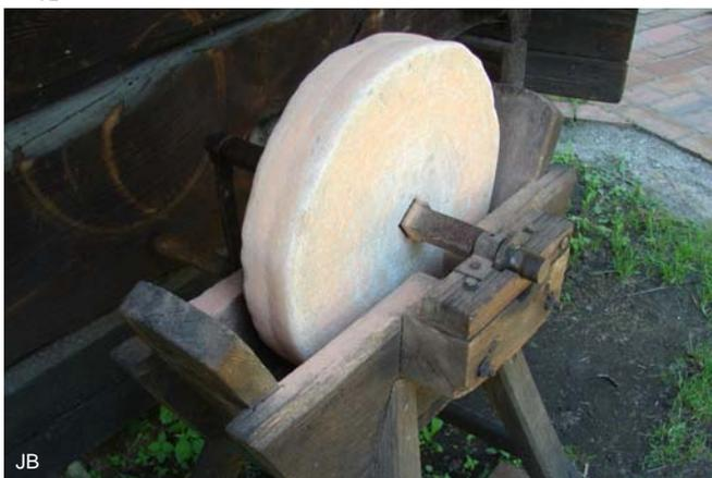
A grinding wheel is a stone-like material to grind or sharpen tools, or to grind anything. A grinding wheel can simply be a sandstone, for example Bentheim sandstone, on which knives are sharpened. Often it is a circular disk, which must be rotated by hand or is used in a grinder.
