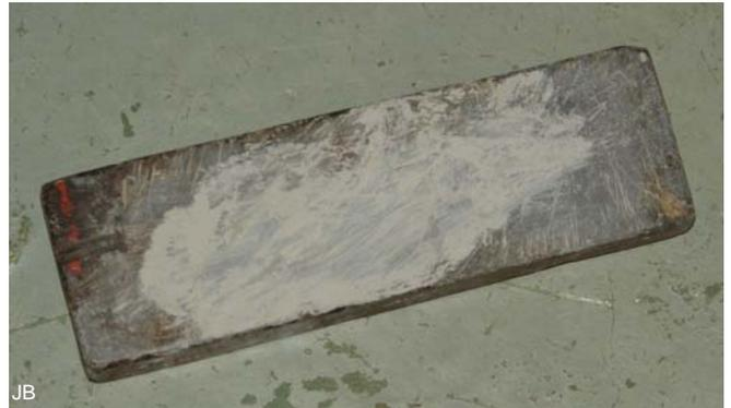
1) Whetstone. Although chisels are made of hardened and tempered steel, they wear in use. Proper maintenance of the tool is necessary. In normal use, occasionally simply use a fine stone or a sharpening steel for the blades.
