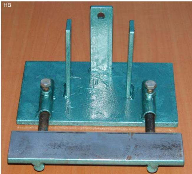
The Aldi (supermarket) grinder has 3 mounting holes of M 8. The stand for the grinder is made of some old iron from my junkyard. Make sure the tool rests perpendicular to the cutting surface. All that's missing now is the dust extraction. See also page 50 of the catalogue: [http://www.beeldhouwwinkel.nl/catalogus\\_2011.pdf](http://www.beeldhouwwinkel.nl/catalogus_2011.pdf)
