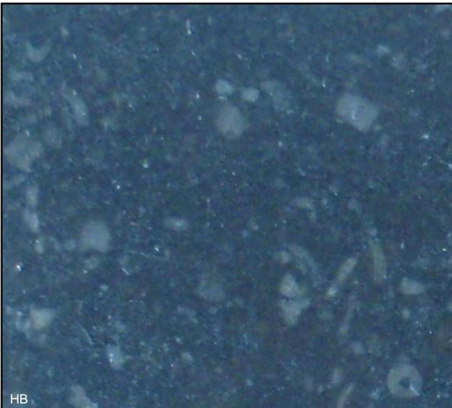
C600 = satin, almost polished, smallest possible surface, grinding marks still visible in raking light.
