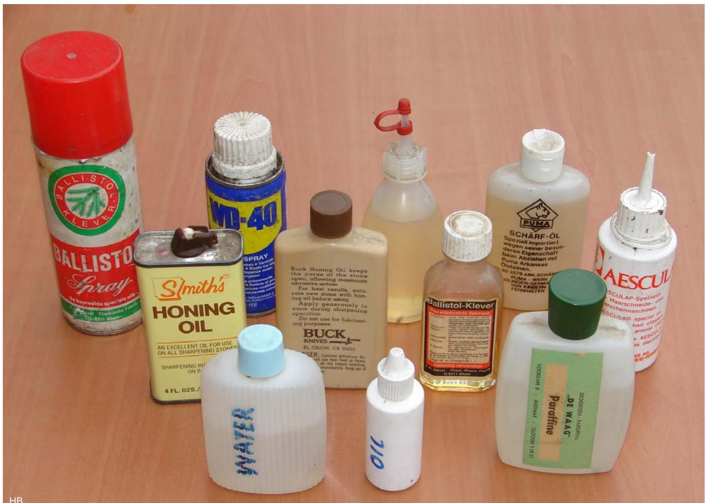
\* Fine stoned need a thinner liquid, since the peaks of the abrasive grains are relatively much lower than with a coarse stone.
