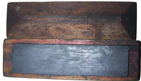
Fine and soft whetstone, also fine sandstone. A finishing stone provides a still finished surface, neither too soft nor too hard. Pretty uniform in composition, the grinding stone does not gnaw the tool. You can compare it to grinding with an artificial grinding stone with a fine grain. Nowadays you can order stones in each grain size, formerly it was just luck, therefore a finishing stone was cherished by the expert because his tools profited when it was used.
