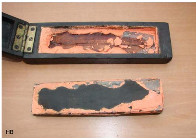
In English whetstone boxes you may find white- and red-lead is mixed in. The reason for the red-lead powder is that it prevents the stone absorbing the linseed oil. Sometimes heated glue of bones is mixed with red-lead powder. I also found a form of Plasticine.
