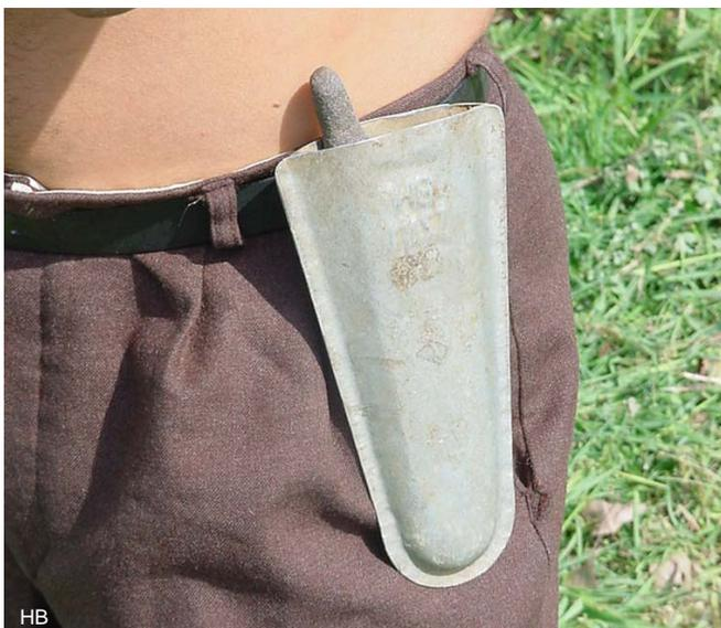
When mowing, the stone or ceramic strickle is worn in a holder on the belt. The holder contained water to keep the stone moist. There are many variations on this subject of wood, cow horn and brass.
