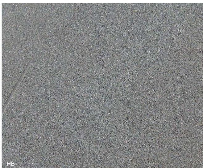
After cleaning it was a very fine engineers stone of SiC (silicon carbide).
