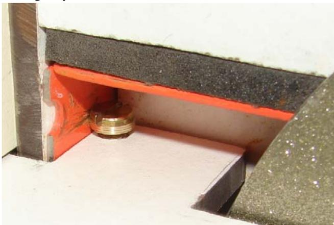
The table is a little bit diagonally mounted to keep the water nearby and can be made square by 2 brass screws M5.
