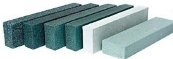
2) Abrasive. A rubbing stone is used when sculpting and takes the shape of the object to sand. Size usually is 25 x 50 x 200 mm, weight about 500 g. Available in 36 grit, 60, 80, 120 and 220.
