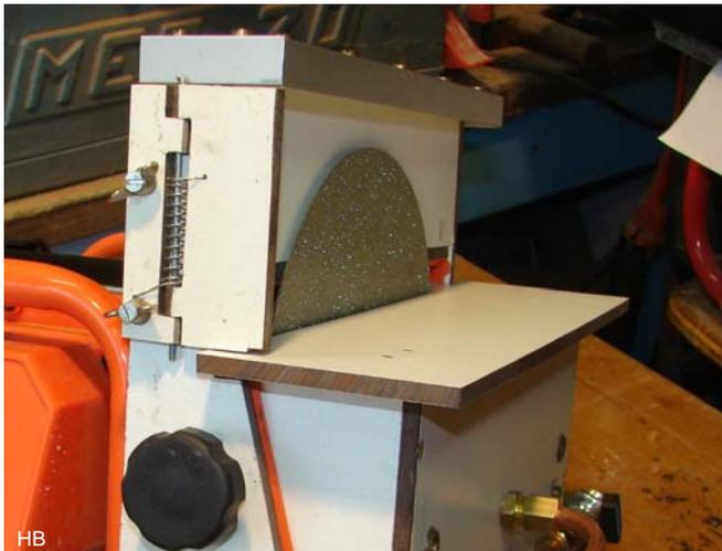
The diamond discs should be water-cooled to ensure that the disk will last long. There is needed very little water and the speed creates a mist of water. In order to prevent the water from being thrown far away, there is arranged a spring-loaded valve so that even long stone can be grinded. Without valve the water came up to 2 meters. At the top is an aluminum angle of 15 x 15 mm. This bends the water downwards so you will become not too wet during grinding.
