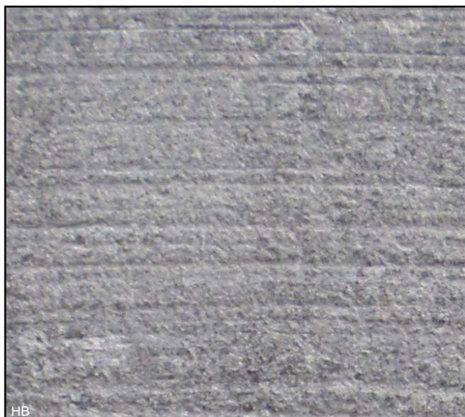
C60 = coarse, abrasive perceptible trace, colour and structure barely visible.
