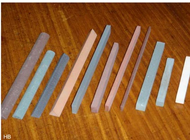
Sharpening files are regularly used by both the jeweller and in machine technology. They exist in natural materials and ceramics made of corundum and silicon carbide. A set consists of coarse, medium and fine in square, triangular, circular, semicircular, 6 x 100 to 20 x 200 mm.
