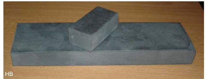
Slurry stone, used with slate to produce a "milky" grinding paste that gives a fast result with a dull surface as a result.
