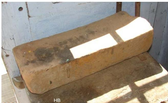
2) In one way or another the edge of a chisel got blunt, then it is sharpened on a sandstone, which grit may be not too fine nor too coarse. Sometimes a sliding stone is used instead of a whetstone. Sliding stones usually have a more or less rectangular shape. They can be purchased at a hardware store, but usually one can get a discarded piece of a grinding stone at be a carpenter.
