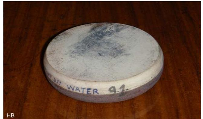
A round, in this case artificial corundum sharpening stone used in machine technology. Similar to the stone used for axes. The name is also used for a circular grinding wheel for a grinder.
