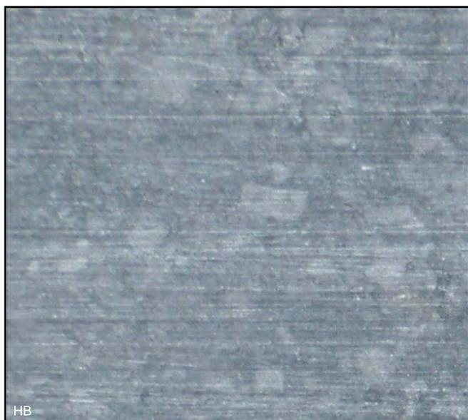
C90 = medium, from top visible grinding marks, rough structures visible, pale colour.
