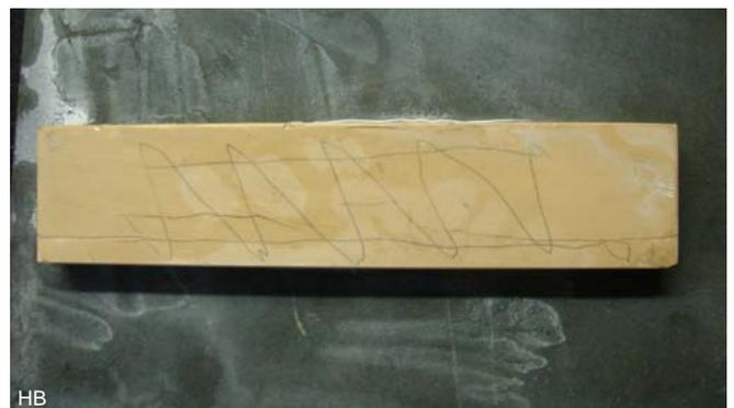
The drawing shows that the stone is a still a little hollow, therefore repeat the operation.
