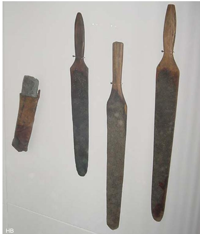
1) A strickle: lath pasted with a coarse abrasive material. Previously, the sand used for the lath was glued to it. Sometimes the manufacturers painted the sand. Today silicon carbide is generally used. Is known by many names.
