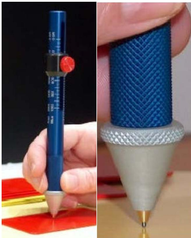
*Hardnesspen Labomat of SP0010. A pocket instrument for testing the hardness and wear -/ scratch resistance of the materials. Tungsten Carbide a point is drawn over the surface with a predetermined constant pressure.*
