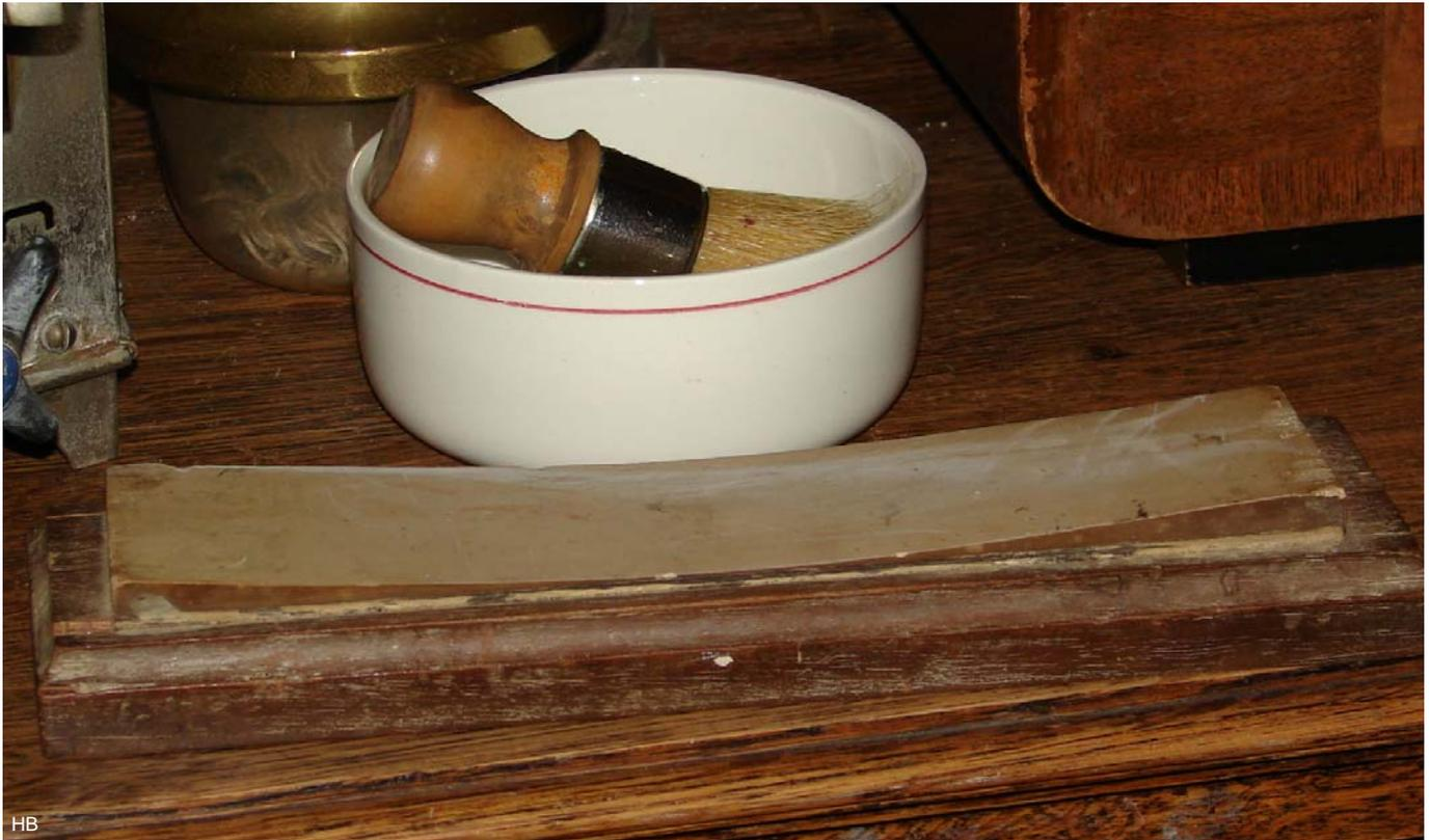
On this stone many razors are sharpened and it is nearing the end of its life. Razors still can be sharpened in this way but not a chisel or planer. You need a flat stone so the cut will be plane.
