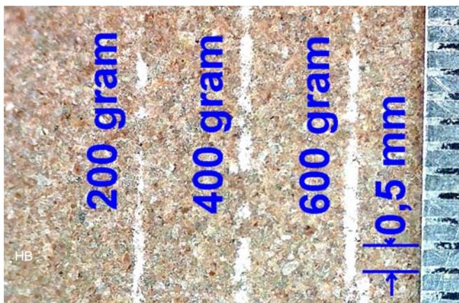
These scratches are made on a Rozsutec. The pressure is increased until after wiping a scratch with a width of 0.3 mm is created.
